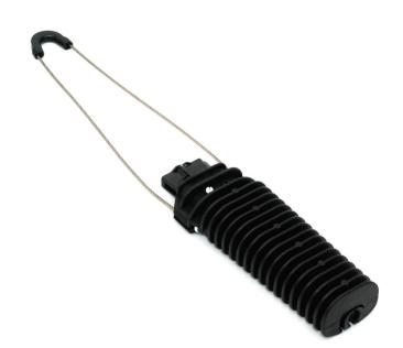
I-T1801.PA-SH cable anchor clamp has been designed to ensure the rapid, simple and secure fastening of ADSS fibre optic aerial cables in a range of diameters from 10 to 16 mm. Anchor clamp consists of removable stainless steel bail, UV resistant plastic wedges and body. The automatic, conical tightening system provides no additional tools for installation and considerably reduces assembly time.
